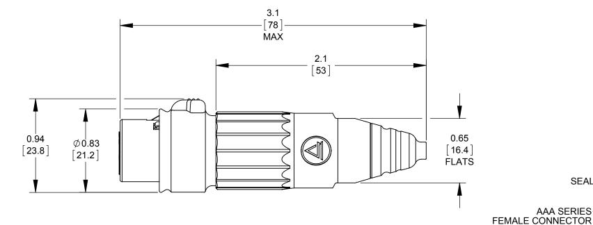
FINISH: -**BLANK** - NICKEL HOUSING, LATCH, & HANDLE/ **GREEN INSERT** B - BLACK HOUSING, LATCH, HANDLE, & INSERT CONTACT PLATING: **BLANK** - SILVER **AU** - GOLD CABLE STRAIN-RELIEF SIZE: **BLANK** - FOR CABLE O.D. 0.150 [3.8 mm] - 0.285 [7.2 mm]
